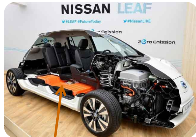
EV battery: Nissan Leaf 24kWh
